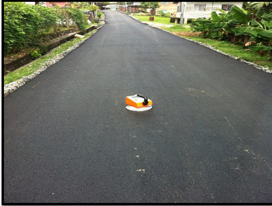
Picture 25: Showing testing of final asphaltic surface – using pavement quality indicator (PQI)
